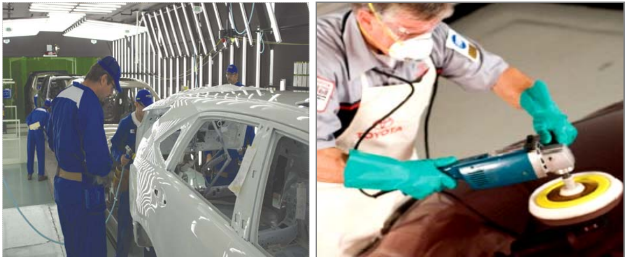
EXAMPLE IMAGES OF TOPCOAT ULTRA-FINE SANDING AND POLISHING TO REMOVE PROCESS INTRUSION DIRT NIBS - FACTORY AND BODY SHOP
